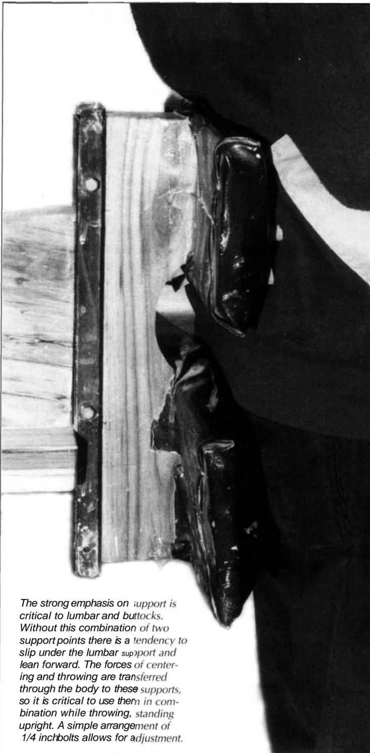
*The strong emphasis on support is critical to lumbar and buttocks. Without this combination of two support points there is a tendency to slip under the lumbar support and lean forward. The forces of centering and throwing are transferred through the body to these supports, so it is critical to use them in combination while throwing, standing upright. A simple arrangement of 1/4 inchbolts allows for adjustment.*
